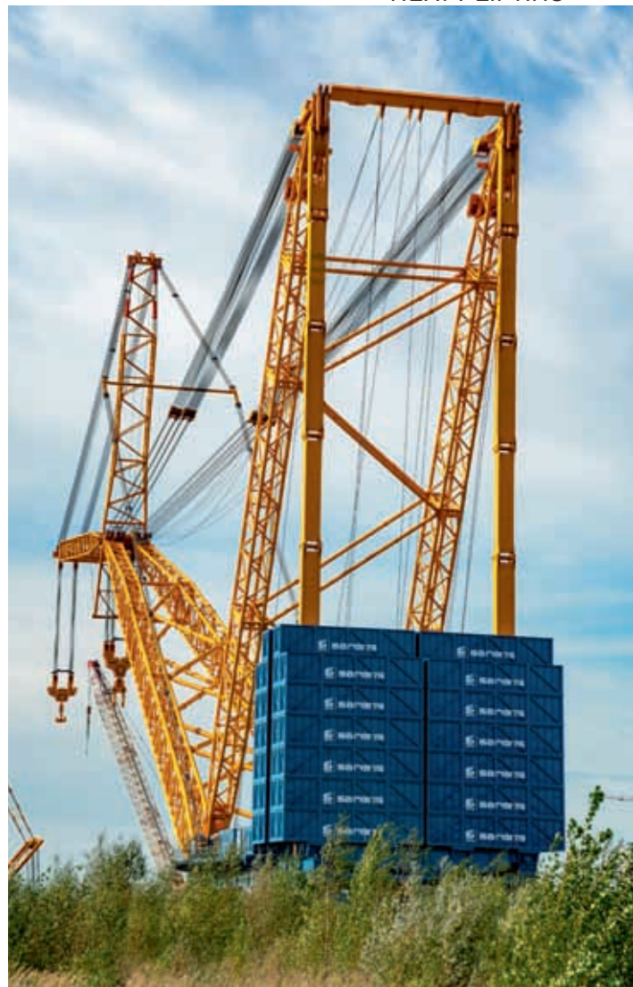
THE SGC-250 HAS 5,200T OF COUNTERWEIGHT, COMPRISED OF REINFORCED CONTAINERS THAT ARE FILLED ON SITE WITH THE AVAILABLE LOCAL MATERIAL OF CHOICE, I.E. SAND.
