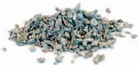
ONE OF THE METALS THAT HEROS EXTRACTS FROM THE WTE BOTTOM ASH IS ALUMINIUM.
