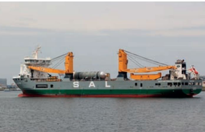
R3ACTOR ON BOARD HEAVY-LIFT VESSEL CALYPSO IN THE SCALDIAHAVEN.
