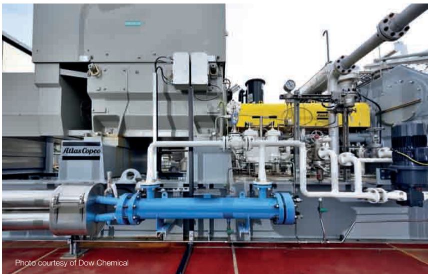
THE STEAM RECOMPRESSION MACHINE THAT WAS BUILT FOR THE PILOT PROJECT AT DOW TERNEUZEN.
