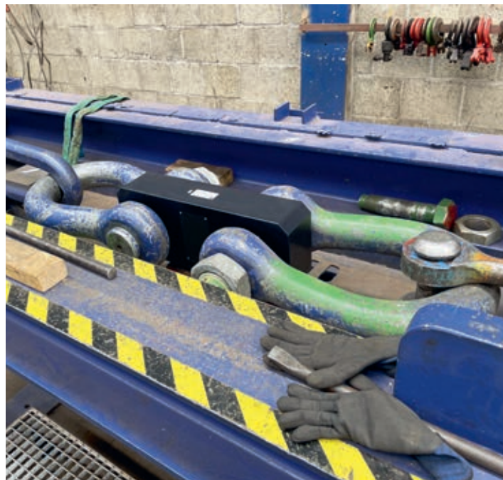
The testing benches can be used for the calibration of even the largest loadcells as well.
