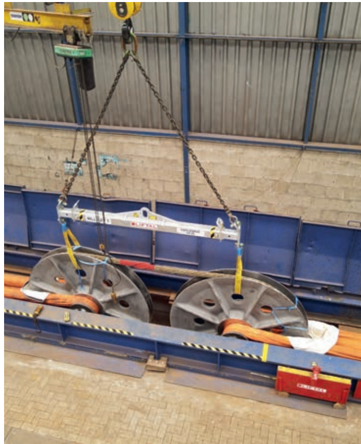
For testing, the Schiedam location now gives Liftal's Test Centre four extra tensile test benches with a capacity up to 2,000t.
