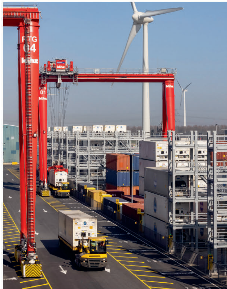
Looking at the horizontal transport of the containers, Kloosterboer wants to improve the efficacy of this, by changing from the current manned to unmanned means of transport.
