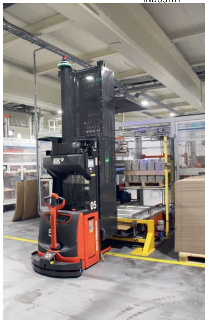
More than half the production lines at Berry Ghent are automated, including the transfer of palletised bottles to the warehouse by AGVs.
