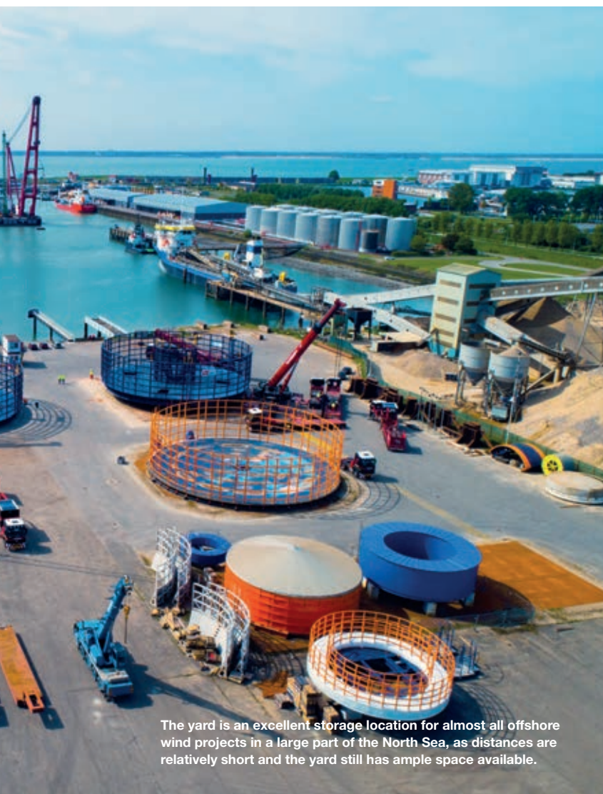
The 9,000t carroussels are the largest liftable carroussels in the world.
