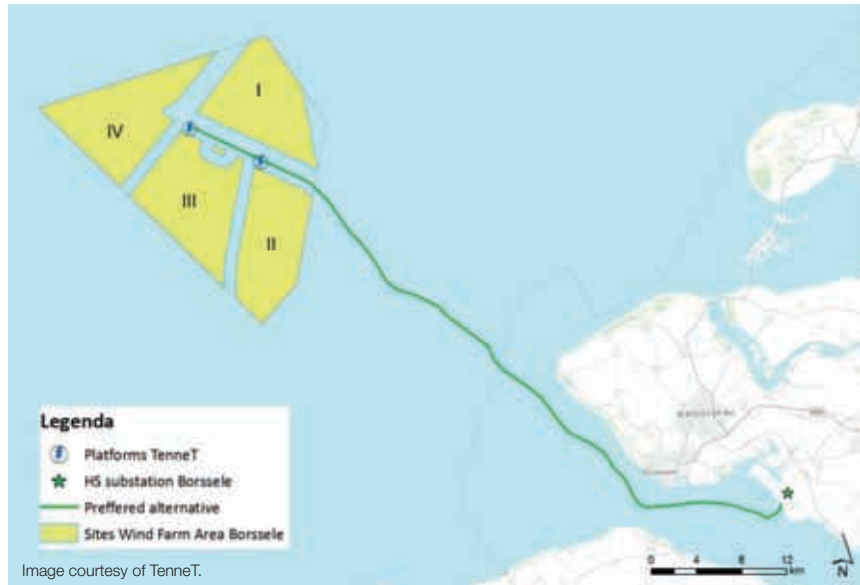
TENNET WILL CONNECT THE BORSSELE WINDFARMS THROUGH TWO PLATFORMS.
